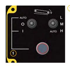
1 The automatic bale feed system helps optimize productivity and provides smooth material feeding through automatic slow down or speed up to maintain a consistent operating PTO and rotor rpm. All this makes it more convenient for the operator to manage the feeding system.
